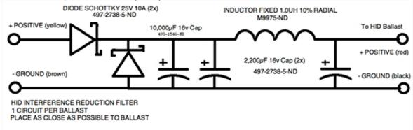
The capacitor-inductor-capacitor "pi" form the lowpass filter. It's tuned to cut anything
