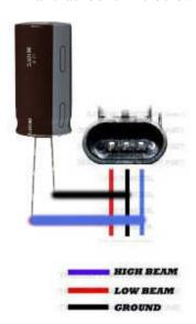
Notice the Center wire is always **Ground**. Depending on which way you look at this plug, one side is High beam and other side Low beam.
